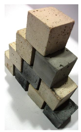
Novacem's cement has already demonstrated performance levels good enough for a range of applications, such as masonry products. The ultimate aim is to produce cement which achieves both price and performance parity with Portland cement – an important step to encourage adoption in the conservative cement industry.
